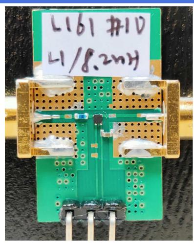
BHWL161 can deliver the GNSS community's lowest NF (0.30 EVB/0.25dB De-Embedded, at ~290K) if implemented with 4-Layer PCB and matched for optimal noise figure instead of best S11.
